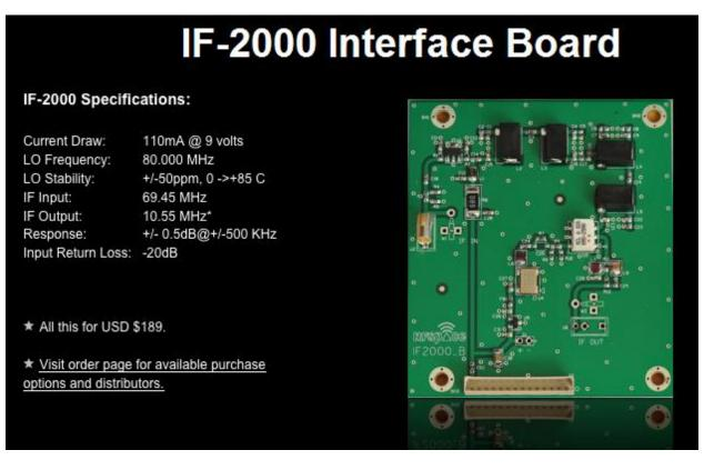
The card's function is to convert the 69.55 Mhz 1<sup>st</sup> IF down to a 10.55 Mhz intermediate IF output which terminates in a BNC pigtail that hangs out of the back of the FT2000.
