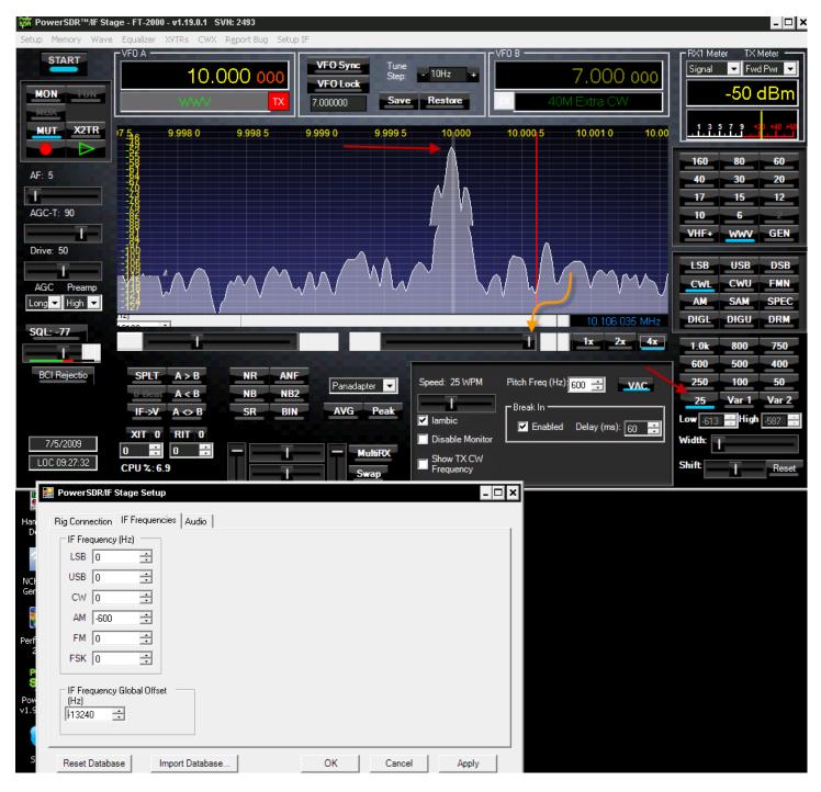
After setting the global for CW, then USB/LSB are setup to operate in the similar manner, adjusting each mode's specific offset to your liking.
