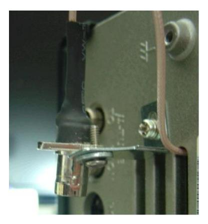
STEP 2: Connect the softrock. The antenna input of the softrock will attach to the IF-2000 BNC dongle on the back of your rig. Power can be supplied from the DC jack on the back of the rig. And the computer sound card will connect to the audio output of the SDR.
