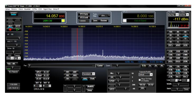
This is more of a visual and aesthetic issue than a functional one. While weak signals near the CF may be lost, the offset between our rig center frequency and the SDR CF means this is typically not a problem at all. Still, it looks a bit odd. <sup>(c)</sup>
