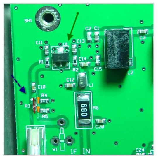
Here we have a close up of the IF-2000 board. The input pad resistors are on the left (blue arrow). And the MC amp is at the top (green arrow).
