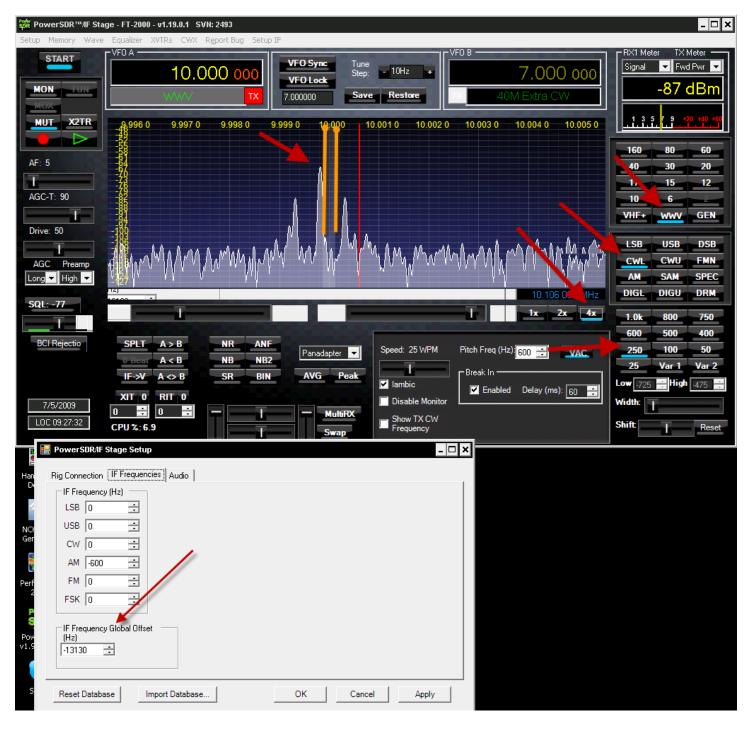
Using the up/down arrows on the left of the IF FREQUENCY GLOBAL OFFSET, adjust the peak of the WWV signal so that it's in the center of the shaded window.
