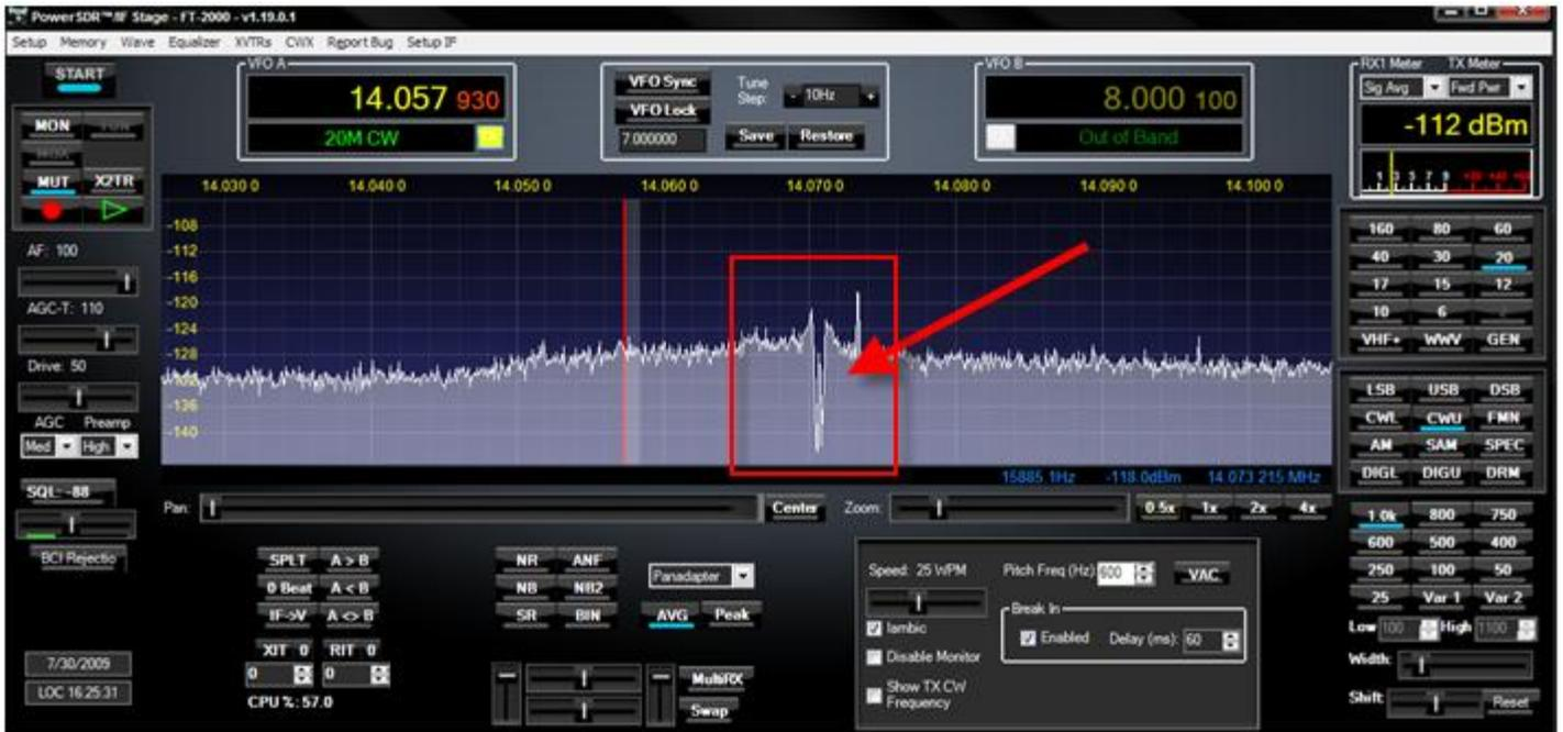
By comparison, here is the LP-PAN under the same conditions. Notice the center frequency dip/hump is completely absent. All the buffering and isolation that's done by the LP-PAN results in a flatter spectrum – even out to 192Khz.
