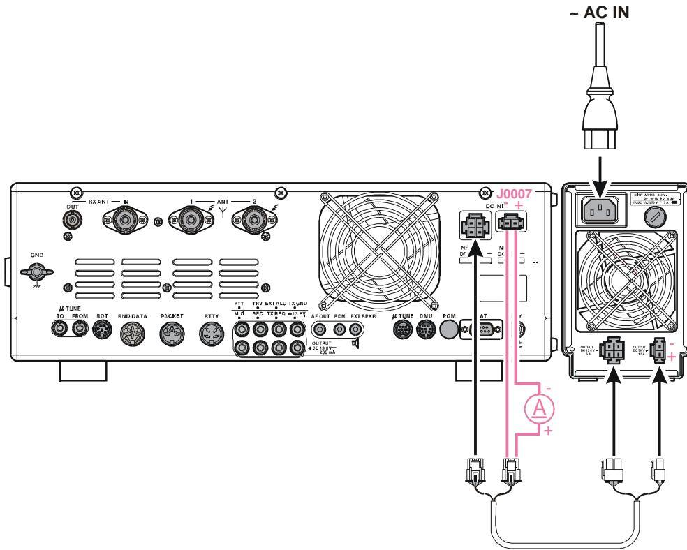
200W PA-B UNIT DC AMMETER CONNECT POINT
